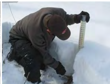
Obtaining snow depth and core sample
