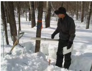
Establish base weight of empty sampling tube
