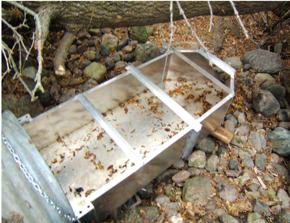
Figure 8. H-Flume Flow Measurement Structure at the Yaggie 2 Site
