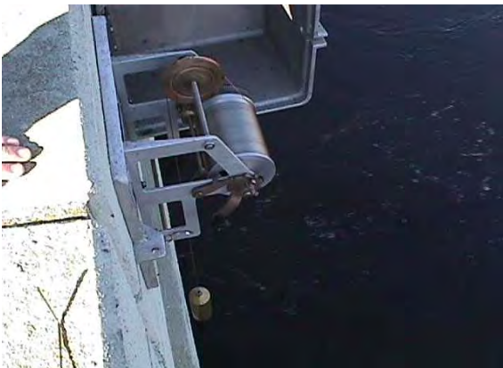
Wire weight stream gage
